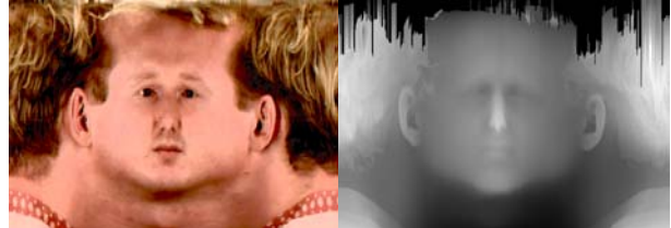
Figure 3: Texture and depth information from the 3-D laser scanner.
