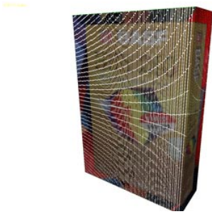
Fig. 2. Illustration of point voxel based occlusion determination. White voxels are misclassified as being occluded although they are actually partially visible. Please note that parts of the background are visible because the voxel volume employed is larger than the extent of the cassette.
