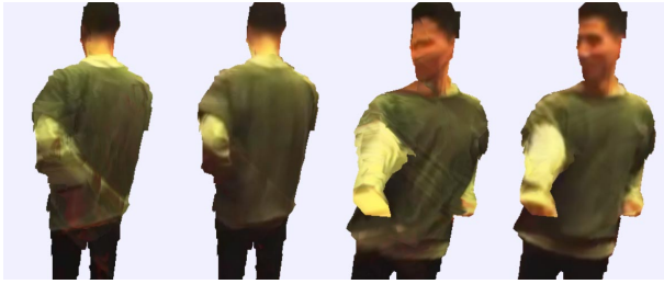
Fig. 6: Rendered views using 4 and 8 textures at same total texture bitrate of 512 kbit/s
