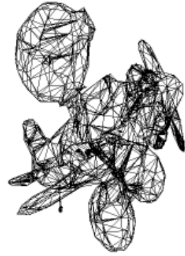
Figure 6: Approximate geometry model, reconstructed from the Airplane light-field images.
