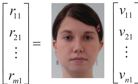
Fig. 1. Representation of a face in 2DPCA using only one vector ( v_1 )
