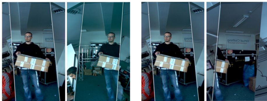
Fig. 9. Stereo content captured by 3D-OMNICAM: left and right view from regular stereo pair at same mirror segment (left) and stereo content from virtual stereo pair across neighbored mirror segments (right).
