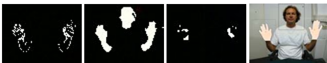
Fig. 7. Result of motion detection, skin-colour segmentation, combination of both and final tracking result of detected hands (from left to right).
