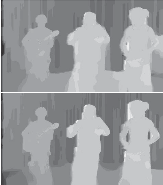
Figure 7: Disparities obtained from the globally optimal geometric image registration step. Top: Result for uncorrected colors. Bottom: Result after registration with the proposed method.
