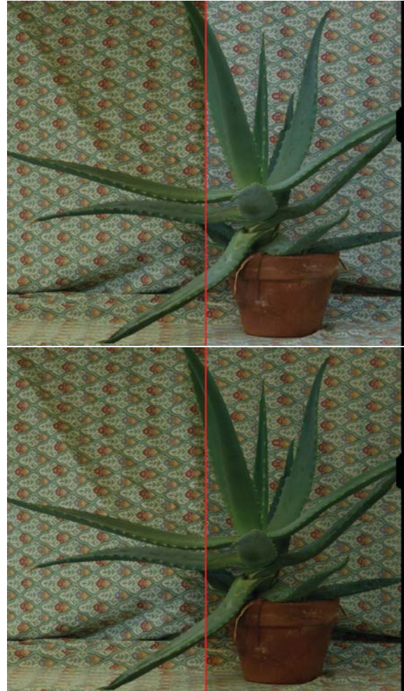
Figure 9: View synthesis based on the scene in figure 8. Both syntheses are composed from the left image of figure 8 on the left of the red line and from the right image on the right of the red line. The synthesis on top is based on original colors and the synthesis on the bottom is performed after a correction with our registration algorithm.
