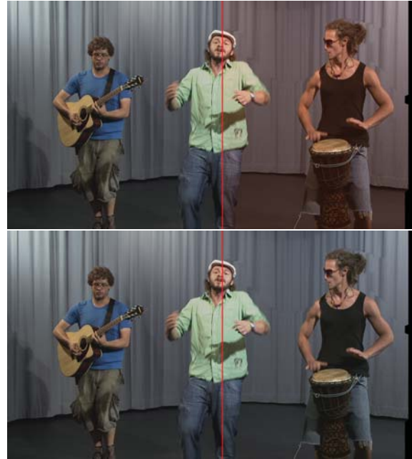
Figure 6: View synthesis based on the scene in figure 5. Both syntheses are composed from the left image of figure 5 on the left of the red line and from the right image on the right of the red line. The synthesis on top is based on the synthetically deviated colors and the synthesis on the bottom is performed after a correction with our registration algorithm.
