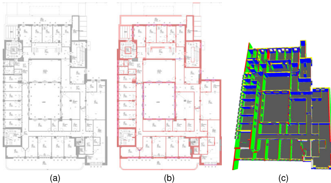
Figure 1: 3D model reconstruction pipeline: a) shows the input floorplan, corresponding to an office building, b) shows an overlay with the extracted, vectorial walls and the detected doors and windows and c) shows a view of the reconstructed 3D model.
