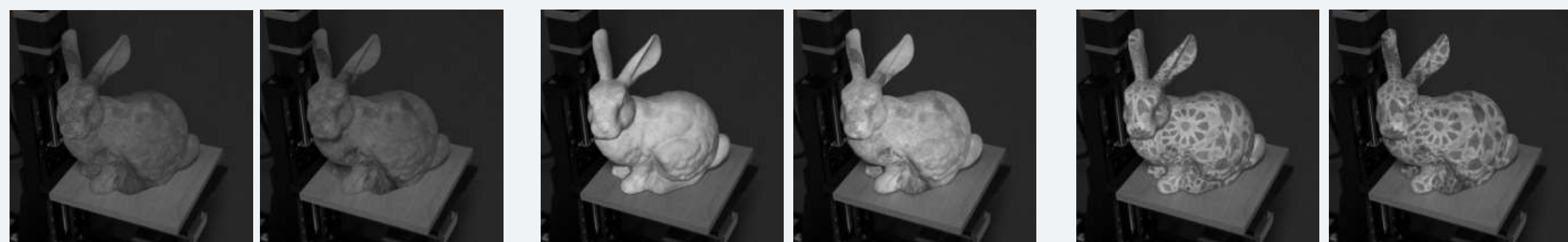
Synthetic rendering vs. camera image for ambient illumination, white and texture projection (from left to right).
