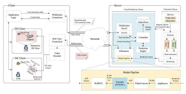
Figure 3 - Overview of cloud-based volumetric streaming framework.
