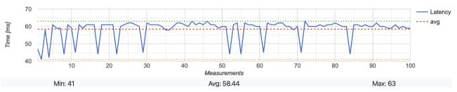
Figure 4 - Results of our motion-to-photon latency measurements.
