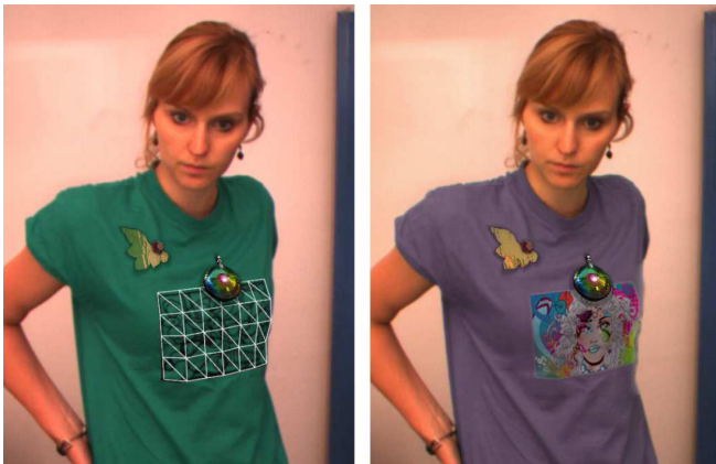
Fig. 6. Two augmented jewel rendering modes combined with cloth recoloring and texture overlay. The center jewel is created by image-based rendering while the left brooch is explicitly modeled.
