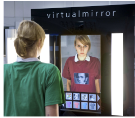
Fig. 1. The Virtual Mirror system replaces color and texture of a t-shirt in real time.
