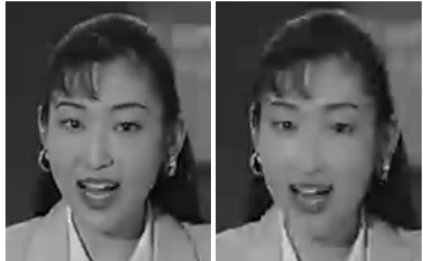
Figure 4: Sample reconstruction for “akiyo”, CIF, 15 Hz, at a bit-rate of 16 kbit/sec. Left: TML4 using proposed entropy coding. Right: original TML4 using UVLC.
