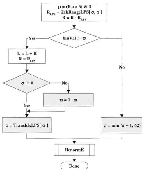
Fig. 8. Flow diagram of the binary arithmetic encoding process including the updating process of probability estimation (in gray shaded boxes) for a single bin value ( $binVal$ ) using the regular coding mode.
