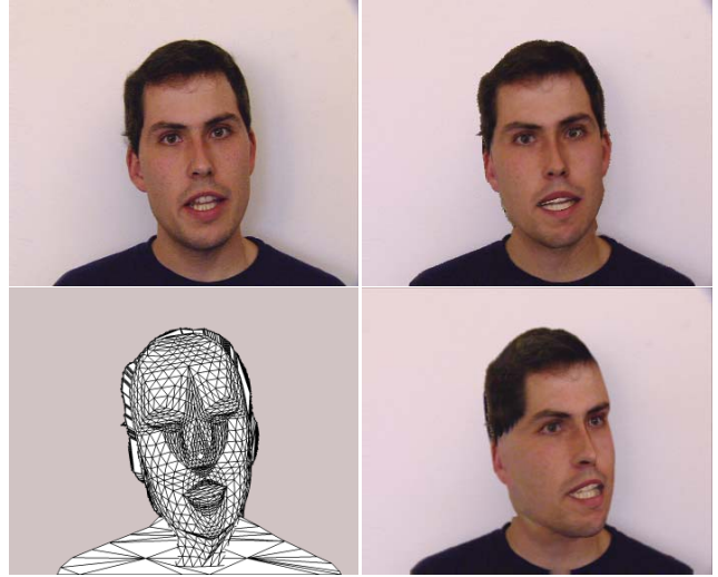
Fig. 3. Upper Left: One original frame of sequence Peter . Upper Right: Textured 3-D head model with FAP's extracted from the original frame. Lower Left: Wire-frame representation. Lower Right: Synthesized frame with head rotated additional 20 degrees compared to the original, showing artifacts at the silhouette.
