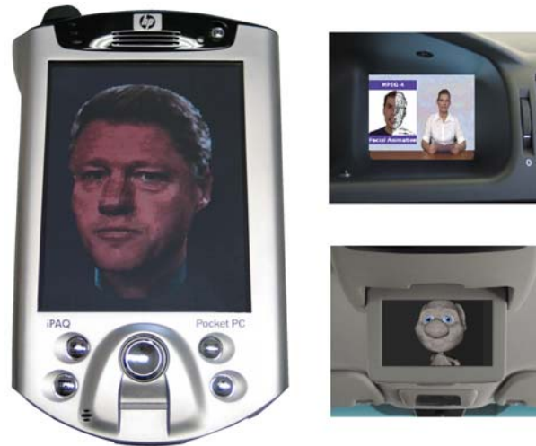
Figure 7: Different Human-Machine interfaces. (left) real-time 3D render engine implemented on a mobile communicator, (middle) in car display units for information and entertainment.
