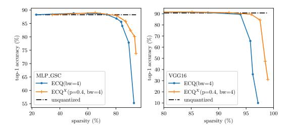
Figure 7: Resulting model performances, when applying ECQ vs. ECQ<sup>x</sup> 4 bit quantization on MLP\_GSC (left) and VGG16 (right). Each point corresponds to a model rendered with a specific  $\lambda$  which is a regulator for the entropy constraint and thus incrementally enhances sparsity. Abbreviations in the legend labels refer to bit width (*bw*) and target sparsity (*p*), which is defined in 4.2.
