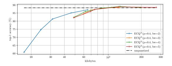
Figure 9: Resulting MLP\_GSC model performances vs. memory footprint, when applying ECQ<sup>x</sup> with 2 bit to 5 bit quantization.
