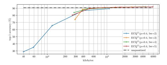
Figure 10: Resulting VGG16 model performances vs. memory footprint, when applying ECQ<sup>x</sup> with 2 bit to 5 bit quantization.
