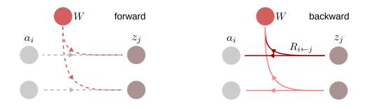
Figure 3: LRP can be utilized to calculate relevance scores for weight parameters W, which contribute to the activation of output neurons  $z_j$  during the forward pass in interaction with data-dependent inputs  $a_i$ . In the backward pass, relevance messages  $R_{i \leftarrow j}$  can be aggregated at neurons / input activations  $a_i$ , but also at weights W.
