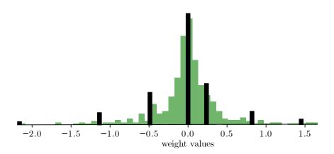
Figure 2: Quantizing a neural network's layer weights (binned weight distribution shown as green bars) to 7 discrete cluster centers (centroids). The centroids (black bars) were generated by k-means clustering and the height of each bar represents the number of layer weights which are assigned to the respective centroid.
