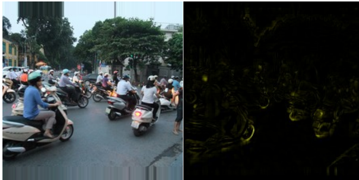
Fig. 1: An image of motor scooters in a complex background and an explanation computed by layer-wise relevance propagation [1] for a classification achieved by the BVLC reference classifier of the caffe package [13].
