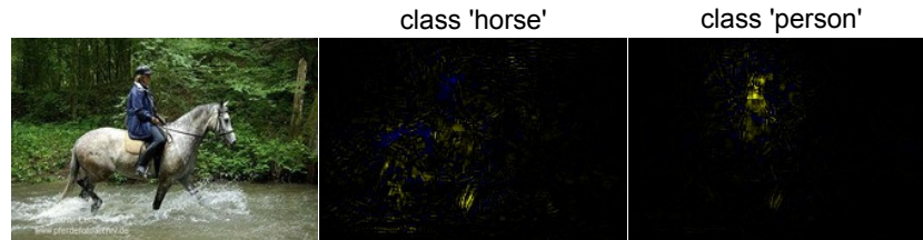
Fig. 6: Explanations are computed by layer-wise relevance propagation [1] for a classification achieved by a classifier trained for multi-label recognition on PASCAL VOC2012. Middle column shows explanation for class horse. Right column shows explanation for class person. Note the shift of focus depending on which object class is to be explained.
