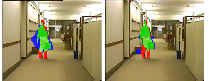
Fig. 3: Tracking accuracies of [3] (left) and the proposed approach (right) in frame 51 of the Hall Monitor sequence. Green, blue, and red colors denote true positives, false positives, and false negatives, respectively.
