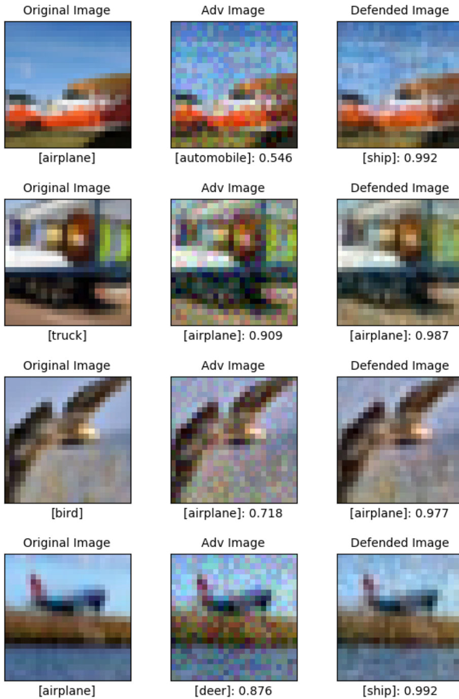
Figure 5: The images are ordered from left to right as the original image, adversarially perturbed image and the defended image. Given below each image are the predicted class label and its corresponding probability of prediction for the respective class
