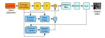
Fig. 1: General diagram of HEVC decoder
