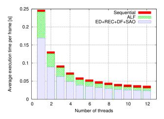
Fig. 5: Breakdown of execution time for class A sequences
