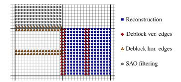
**Fig. 2**: The decoder stages are applied on different adjacent LCUs to maintain the kernel dependencies. Each square represent a  $4\times4$  pixels.
