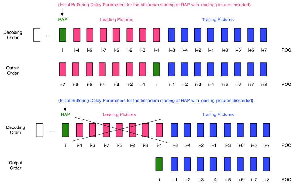
Figure 5: Selection from alternate sets of initial buffering parameters at a RAP picture
