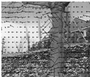
prediction signal \hat{s}[x, y, t] with motion vectors
