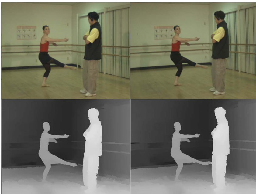
Fig. 7. Example for depth enhanced format: two view plus depth format for the Ballet set.
