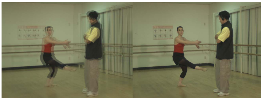
Fig. 5. Intermediate view synthesis from color-only camera data with alias (left) and from color with 8-b depth values without alias (right) for the Ballet set.
