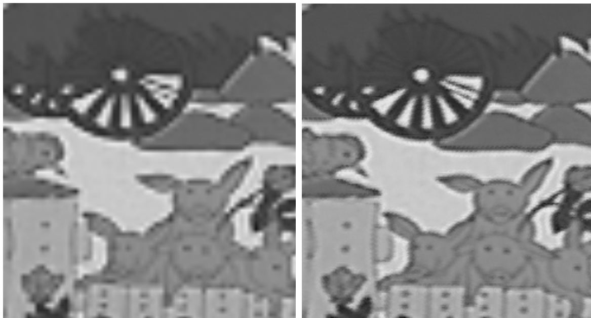
Fig.5 Details from images with 16 times the resolution of the original, for frame no. 150 of sequence Mobile & Calendar, left: bilinear interpolation from original image, right: high-resolution mosaicing.
