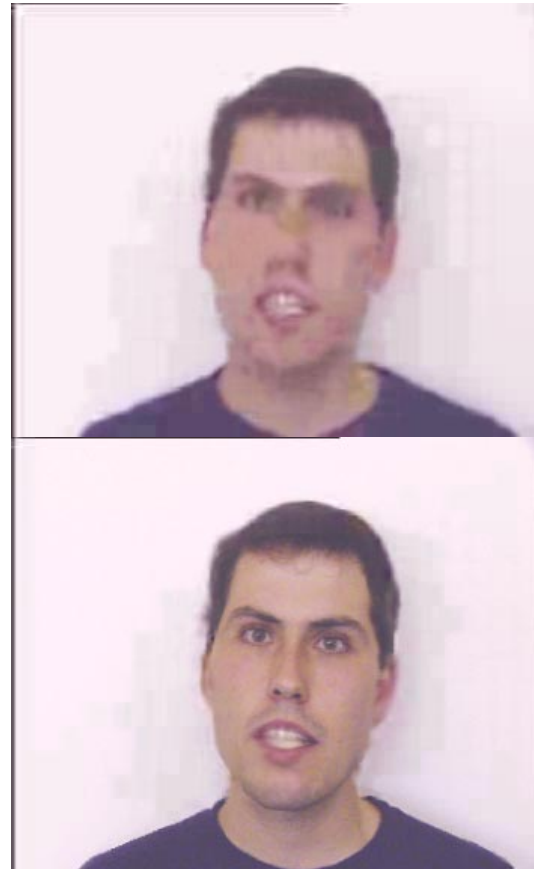
Figure 6: Frame 120 of the Peter sequence coded at the same bit-rate using the TMN-10 and the MAC, upper image : TMN-10 (33.88 dB PSNR, 1680 bits), lower image : MAC (37.34 dB PSNR, 1682 bits).
