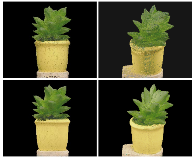
Figure 10. Reconstructed views of the plant . The lower images show the results obtained when considering extended voxels. The upper images show the results for point voxels.
