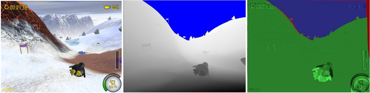
Figure 1: Input frame-buffer from game (left), corresponding depth map with blue colored skybox region (middle) and difference image of input frame-buffer and per pixel prediction based on previous frame (right)
