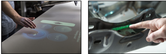
Figure 3. Interaction in a collaborative human-robot inspection by projector-based AR. Left: Touchless interaction with a projective interface. Right: Gesture based object interaction with a welding line marked by the projector.
