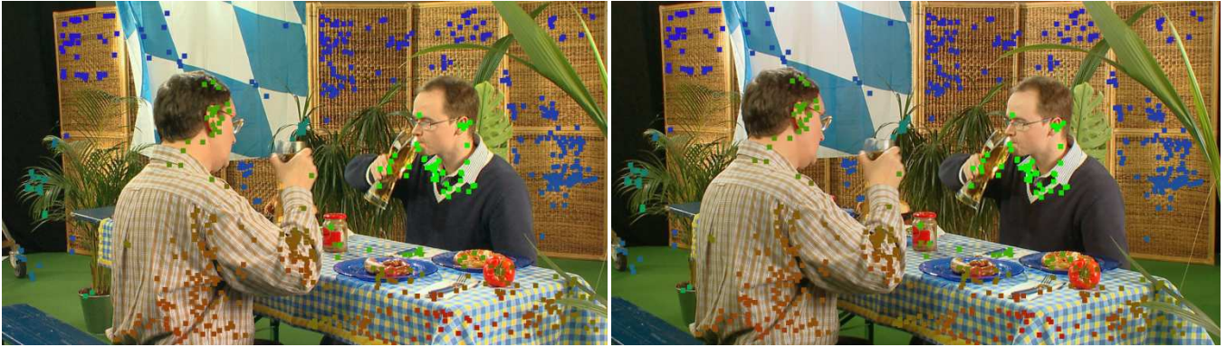
Figure 15: Screenshot of the real-time stereo matching application. One can see that the scene contains objects in different distances to the stereo camera. The matched feature points are coloured according to their horizontal disparity, brown for near objects, blue for far objects in blue. Apparently, no outliers are visible. The full sequence is available as supplementary data. The original resolution used for the matching was 960x540 pixel.
