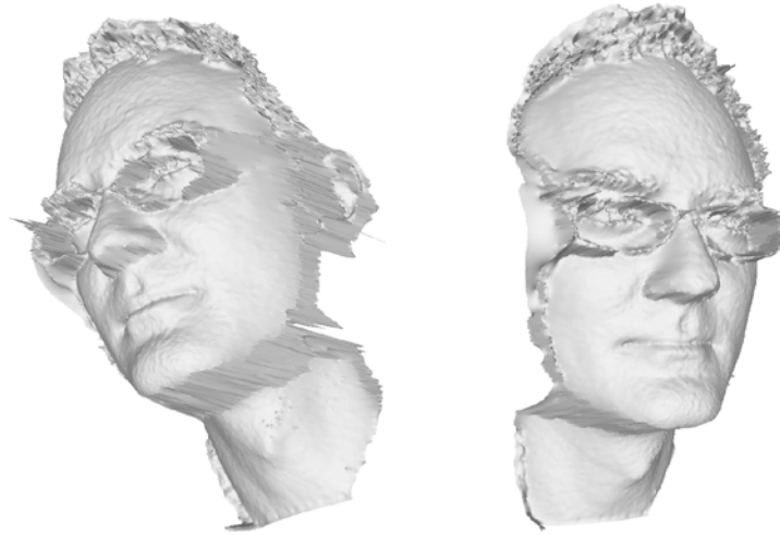
Fig. 8: Obvious difficulties in reconstructing the fine structure of the spectacle frame and subtle errors introduced by the refraction of the lenses (distorted eye regions)
