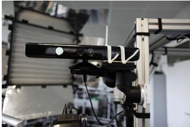
Fig. 2: Kinect video depth sensor mounted on the prototype
