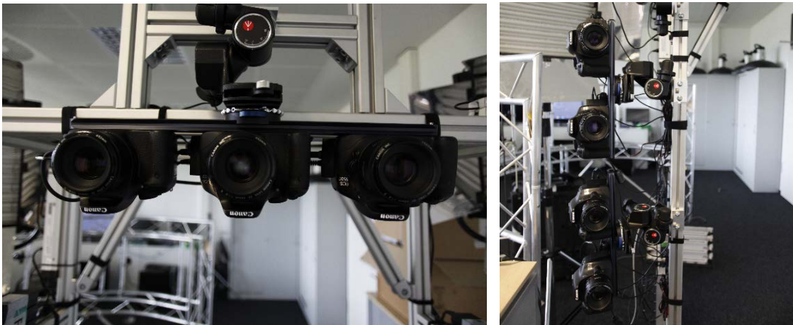
Fig. 5: D-SLR cameras mounted on the prototype
