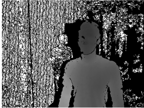
Fig. 3: Depth output of the Kinect Sensor
