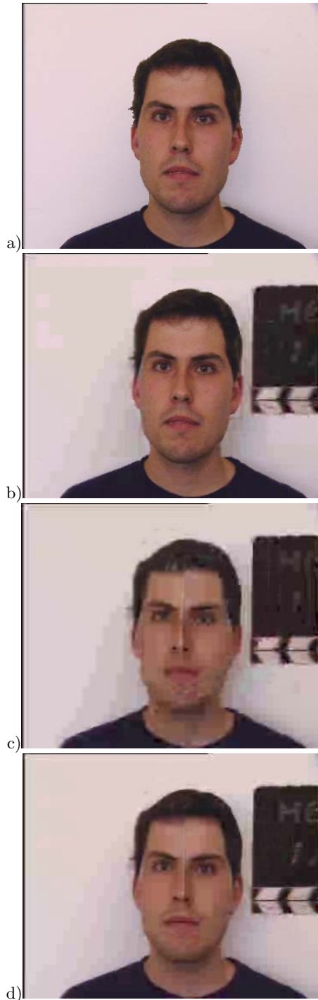
Figure 7: Frame 54 of the sequence Clapper Board . a) Model frame with missing clapper board; b) MAC, 36.1 dB, 2900 bits; c) TMN-10 with same bit-rate as MAC, 32.7 dB, 3200 bits; d) TMN-10 with same PSNR as MAC, 36.0 dB, 5800 bits.
