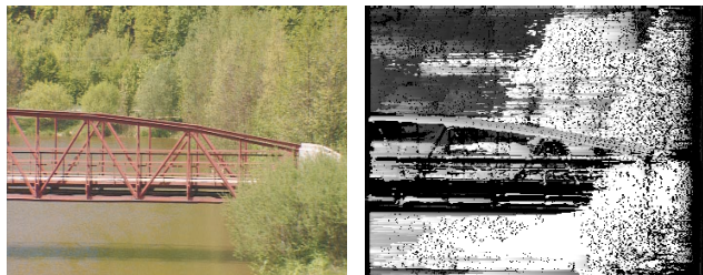
Fig. 8. "Bridge", real sequence with linear horizontal camera movement, left) original image, right) estimated depth
