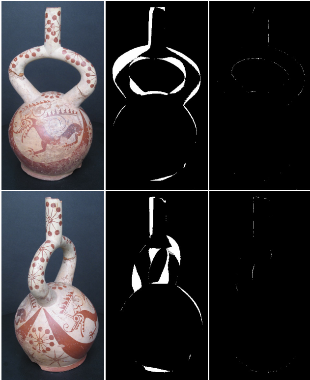
Fig. 5. Silhouette optimization with no initial pose information from calibration. Middle: Large initial silhouette error; right: significantly reduced deviations after optimization.
