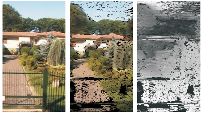
Fig. 8. 3D reconstruction of the 'House'-sequence, (left) original image of the sequence, (middle) reconstructed 3D model, (right) reconstructed depth map
