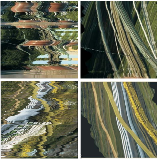
Fig. 7. Horizontal slices in the image cube illustrate the structure of the ICTs, (left column) before parameterized correction, (right column) afterwards. top row) 'Neptun'-sequence, bottom row) 'Park'-sequence.
