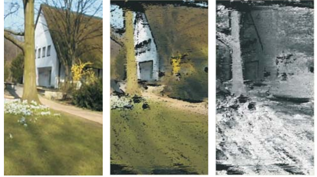
Fig. 9. 3D reconstruction of the 'Park'-sequence, (left) original image of the sequence, (middle) reconstructed 3D model, (right) reconstructed depth map
