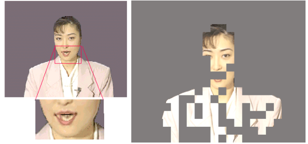
Figure 8: left: model frame 18 of the sequence Akiyo with enlargement of the image region around the mouth, right: corresponding selection mask showing those macroblocks that have been selected from the model frame.
