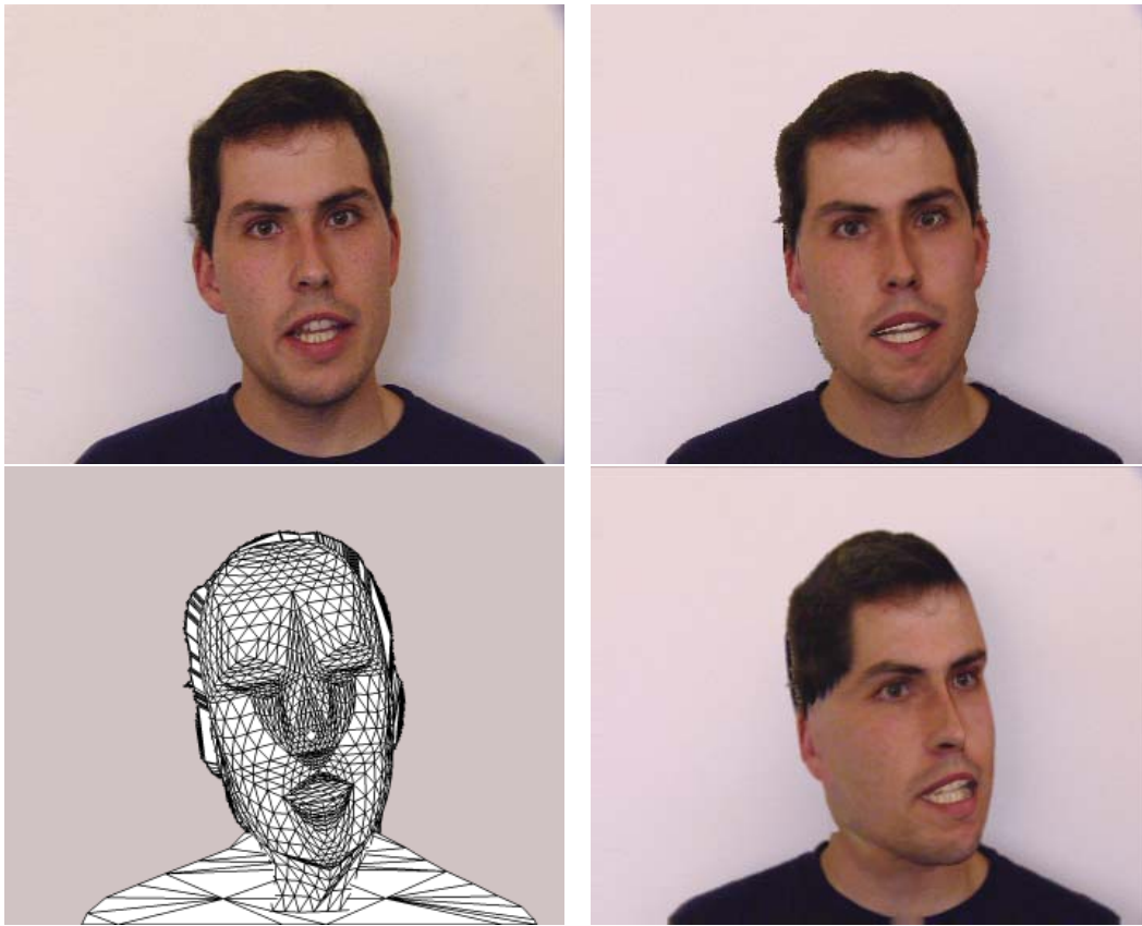
Fig. 4. Upper Left: One original frame of sequence Peter . Upper Right: Textured 3-D head model with FAP’s extracted from the original frame. Lower Left: Wireframe representation. Lower Right: Synthesized frame with head rotated additional 20 degrees compared to the original, showing silhouette artifacts.
