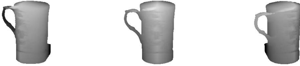
Figure 20: Depth maps rendered from the reconstructed 3-D volume for the same viewing positions as in frames 1, 5, and 9 of the Cup sequence.
