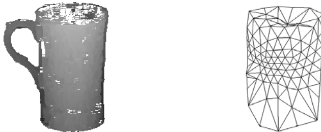
Figure 18: Left: Depth map of frame 5 of the Cup sequence obtained from the structure-from-motion step. Right: Generic shape model after initialization.
