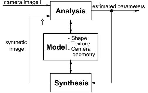
Figure 4: Analysis-synthesis loop of the motion estimation framework.
