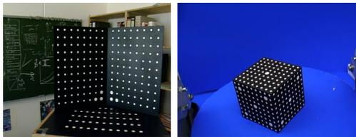
Figure 1: Two different calibration test objects.
