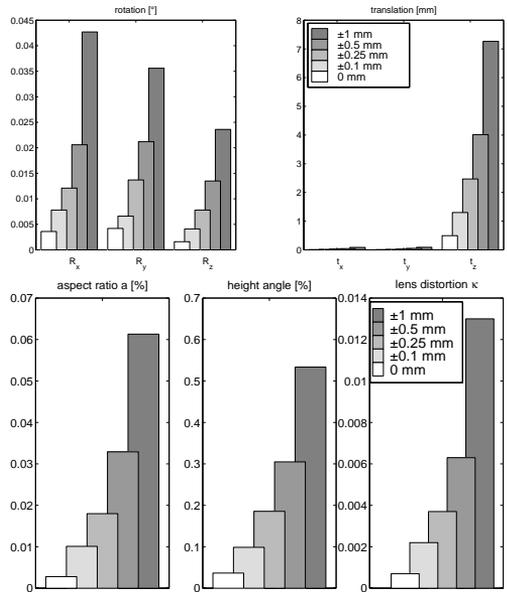
Figure 6: Average absolute error of the estimated internal and external camera parameters for test objects of varying accuracy. Aspect ratio  $a$  and height angle  $\varphi_{height}$  are specified relative to their mean  $\bar{a} = \frac{4}{3}$  and  $\bar{\varphi}_{height} = 0.5$ , respectively.
