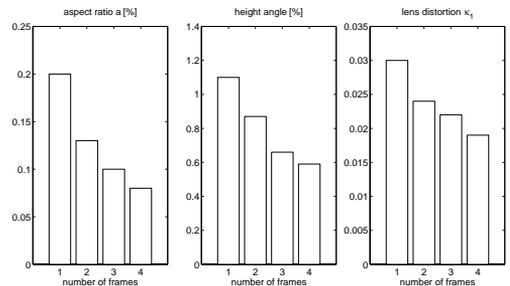
Figure 8: Standard deviation of the internal camera parameters for different numbers of frames used simultaneously in the estimation.
