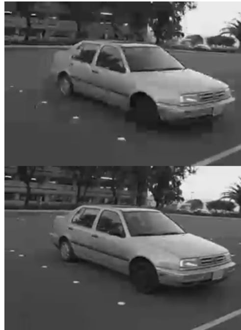
Figure 6. Reconstructed frame 10 of Car using (Top) TML-8.0 (28.5 dB) and (Bottom) MAC (31.5 dB) at 2.0 kbits/P-frame.
