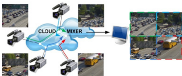
Figure 1: System architecture for video mixing, e.g. traffic video surveillance
